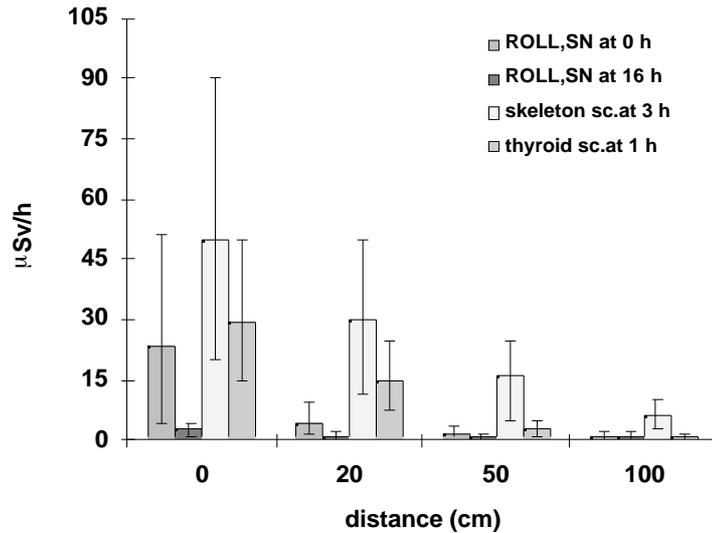
**Fig. 1** Air kerma rate ( $\mu\text{Gy/h}$ ) for SN and ROLL at 0, 20, 50, 100 cm from patient, 0 and 16 h after administration. Values are compared to the air kerma rate after bone and thyroid scintigraphy (dotted bars). Mean values and range over 50 patients.
